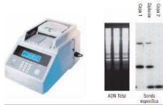
Fig. 4 Thermal cycler for PCR and Southern Blot
